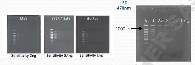
The best sensitivity (1 ng) when MaestroSafe is used combined with Maestrogen's LED Transilluminator.
