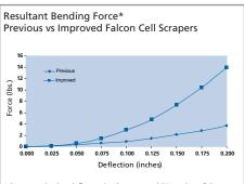
\* Force required to deflect a simply supported 5" portion of the handle 2.5" distal to the handle section: resultant = ('X' force) ('Y' force)
