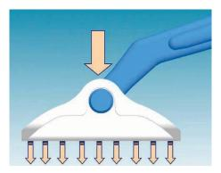
Unique blade design transfers scraping force to the blade edge, allowing it to conform to the scraping surface.
