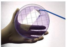
The **Cat. No. 353089** cell scraper has a larger blade to increase cell scraping efficiency in both Falcon dishes and 75 cm<sup>2</sup> flasks.
